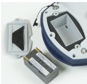
The battery used in the ProMark 800 is a 7.4-V DC - 4600 mAh rechargeable battery. It is a standard model used in many camcorders.
